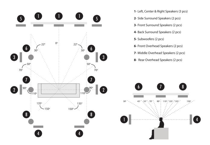
2. The illustration below shows an example of positioning a 7.2.6 system, as reference. (The images in this illustration differ from the actual units for explanation purposes.)
