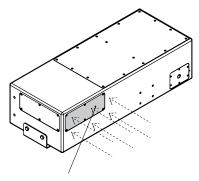
Replace Port components into alternate port location
