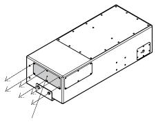
Remove Port components from current port location
