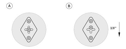
SOUNDBAR WILL SLIDE DOWN 3/8" BELOW THE SCREW HOLE LOCATION
