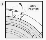
OPEN POSITION: PULL THE METAL LOCK TAB AWAY from the Bayonet Ring, before removing loudspeaker from Bayonet Ring.
