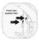
**Note:** If the Bayonet Zip-Clips<sup>™</sup> need to be adjusted or removed, depress the metal tabs along the rail and push up.
