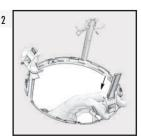
Reach through and **PLACE 2 FINGERS ON THE GROOVES** of the Bayonet Zip-Clip<sup>™</sup> to pull each Zip-Clip<sup>™</sup> down the rail.
