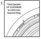
TWIST THE SPEAKER 15 ° CLOCKWISE, until the indicators on both the Bayonet Ring & the Speaker are aligned.
