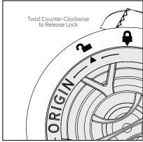
Twist the Speaker COUNTER- CLOCKWISE, so that the arrow on the Speaker Rim, aligns to the "UNLOCKED" Symbol along the Bayonet Ring. Now the Speaker should be unlocked from the ring. Use caution to remove the speaker from the Bayonet Ring, without forcing the lock mechanism.
