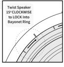
TWIST THE SPEAKER 15 ° CLOCKWISE, until the indicators on both the Bayonet Ring & the Speaker are aligned.
