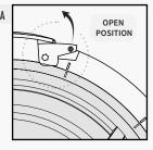
**OPEN POSITION: PULL THE METAL LOCK TAB AWAY** from the Bayonet Ring, before removing loudspeaker from Bayonet Ring.
