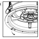
After connecting wires, insert the Speaker into the Bayonet Ring, with the METAL LOCK TAB LIFTED AWAY FROM THE RING.
