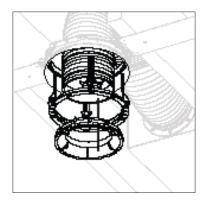
Install the BZ68 bayonet ring. Pull the port tube through the ring, slip the port adapter into the end and tighten the screw on the hose clamp to get a snug, secure attachment.
