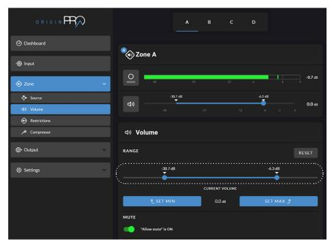
On the device, the end user is made visually aware of the volume range limitation when adjusting the volume level (see below).
