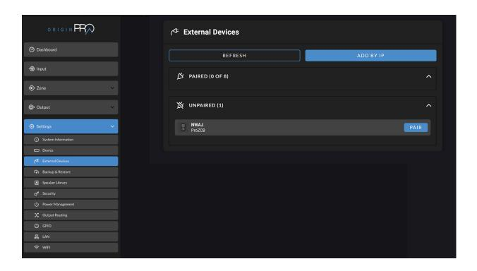
The PROZCB | PROZCW Wall Controller device you are configuring will be displayed under 'UNPAIRED' devices.
